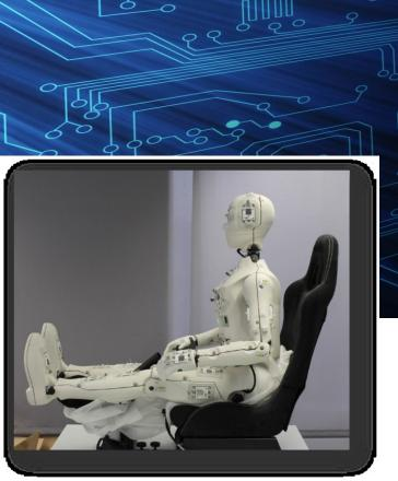
The HVAC manikin was developed by ARRK Engineering to help OEM manufacturers evaluate and measure the passenger thermal comfort and environmental conditions in the automotive industry.
